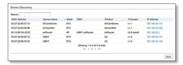
It reports the MAC Address, Device Name, Mode, SSID, Product type, Firmware version, and IP Address for each Ubiquiti device. To access a device configuration through its web management interface, click the device's IP address.
